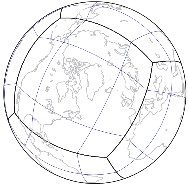
Figure 10. Aerial view showing our second adaptation of the cubed sphere of Ronchi et al. (1996). The black lines identify the boundaries of the six chunks that were apparent also in Fig. 1. The blue lines correspond to the boundaries of the overlapping ‘superchunks’ as discussed in the text.
