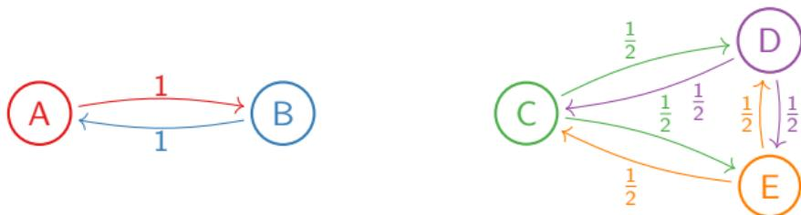
The importance matrix is  $\begin{pmatrix} 0 & 1 & 0 & 0 & 0 \\ 1 & 0 & 0 & 0 & 0 \\ 0 & 0 & 0 & \frac{1}{2} & \frac{1}{2} \\ 0 & 0 & \frac{1}{2} & 0 & \frac{1}{2} \\ 0 & 0 & \frac{1}{2} & \frac{1}{2} & 0 \end{pmatrix}$ . This has linearly independent eigenvectors  $\begin{pmatrix} 1 \\ 1 \\ 0 \\ 0 \\ 0 \end{pmatrix}$  and  $\begin{pmatrix} 0 \\ 0 \\ 1 \\ 1 \\ 1 \end{pmatrix}$ , both with eigenvalue 1. So there is more than one rank vector!
