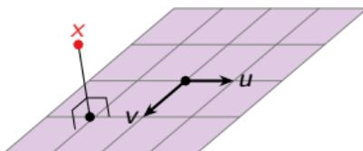
Due to measurement error, though, the measured  $x$  is not actually in  $\text{Span}\{u, v\}$ . In other words, the equation  $au + bv = x$  has no solution. What do you do? The real value is probably the *closest* point to  $x$  on  $\text{Span}\{u, v\}$ . Which point is that?
