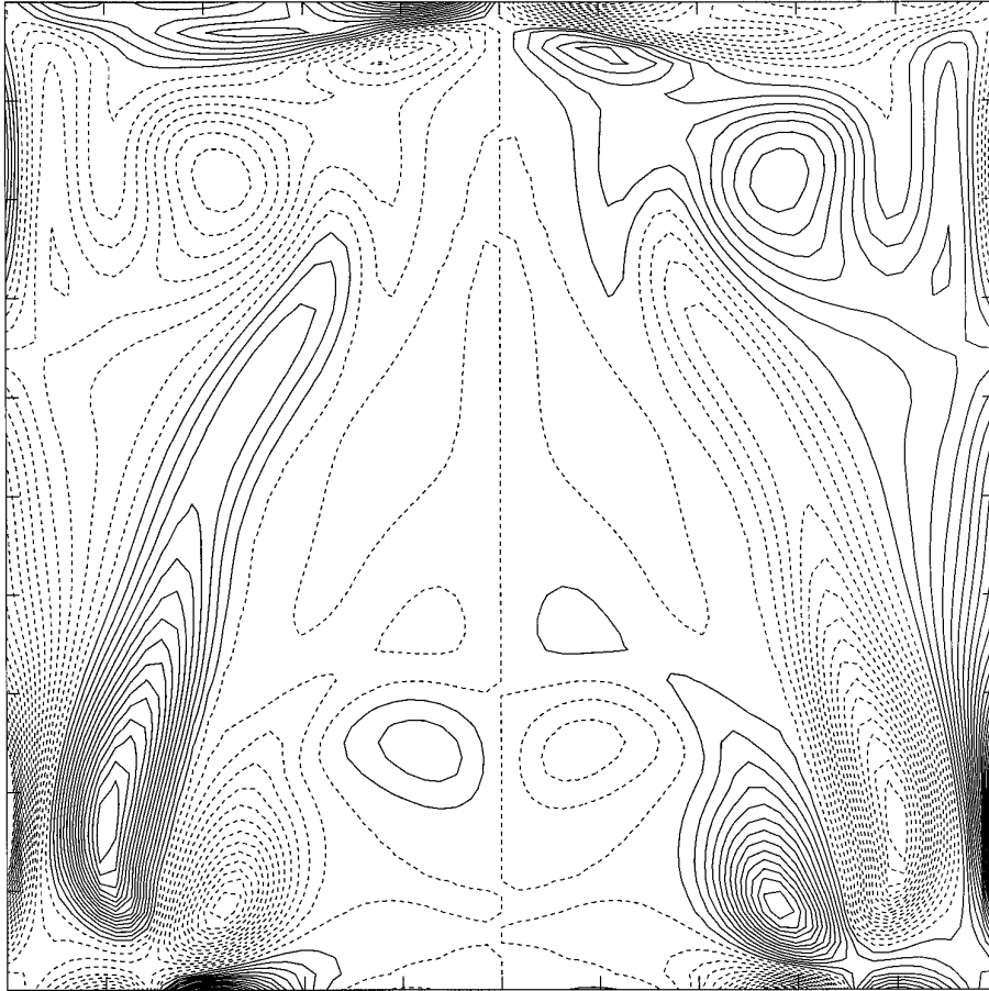
FIG. 10. Contour plot of \omega_1 at the center plane \{x = \frac{1}{2}\} computed using Method B and (4.1). Parameters: Re = 3200 , t = 15 , CFL = \Delta t/\Delta x = 2.5 , \Delta x = \frac{1}{64} .
