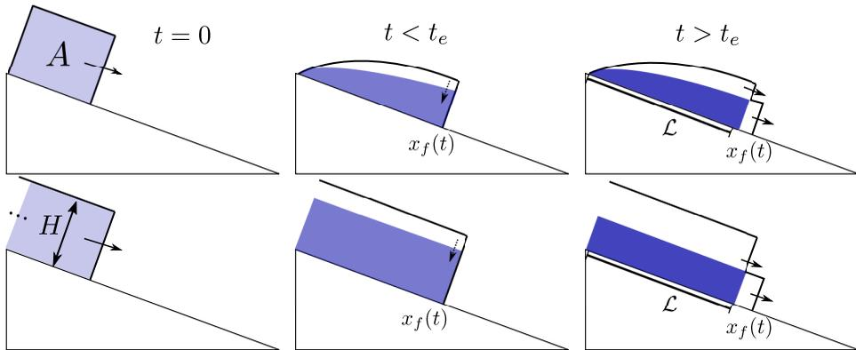
FIGURE 3. In the settled regime, sketch of the model for the ‘transition distance’  $\mathcal{L}$  before the suspension separates into distinct fronts, given either a fixed initial area  $A$  (top) or constant upstream height  $H$  (bottom). The bulk flow is assumed to evolve as well-mixed up to a time  $t_e$  as the particles equilibrate in the  $z$ -direction.
