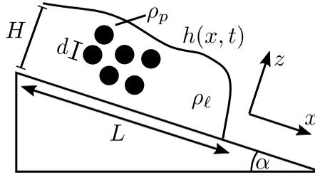
FIGURE 1. Problem diagram: A suspension with particle and fluid densities  $\rho_p$  and  $\rho_l$  with a free surface  $h(x, t)$  and  $\rho_p > \rho_l$  flows under the influence of gravity down an incline at an angle  $\alpha$  from horizontal. The film has a characteristic height  $H$  and length  $L$  with  $H \ll L$ .
